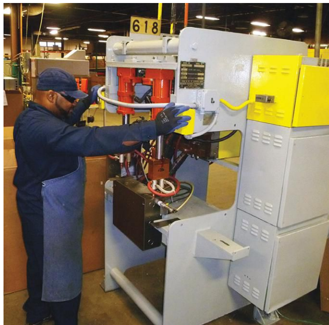
A DureX worker operates a multihead spot welder. Using it increases efficiency by welding four spots in one stroke.
