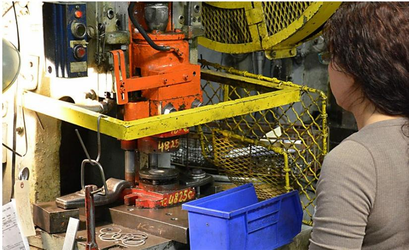
*Tools can also be staged to create a blank before a secondary press is used to form it into a box with another hard tool.*
