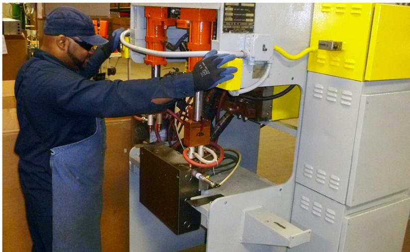
*A DureX worker operates a multihead spot welder. Using it increases efficiency by welding four spots in one stroke.*
